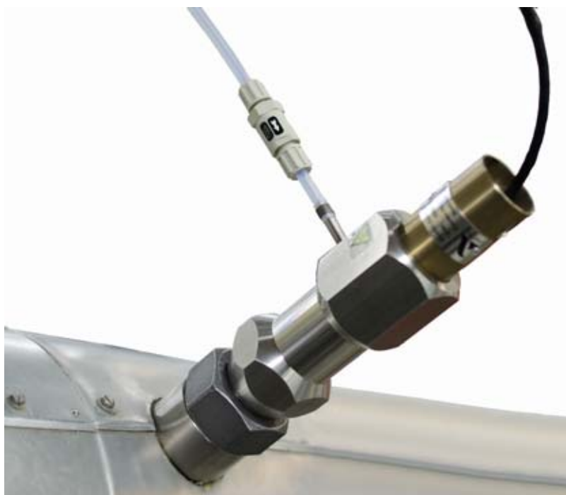
Fig. 8-2 Testing device plugged into flue gas channel
