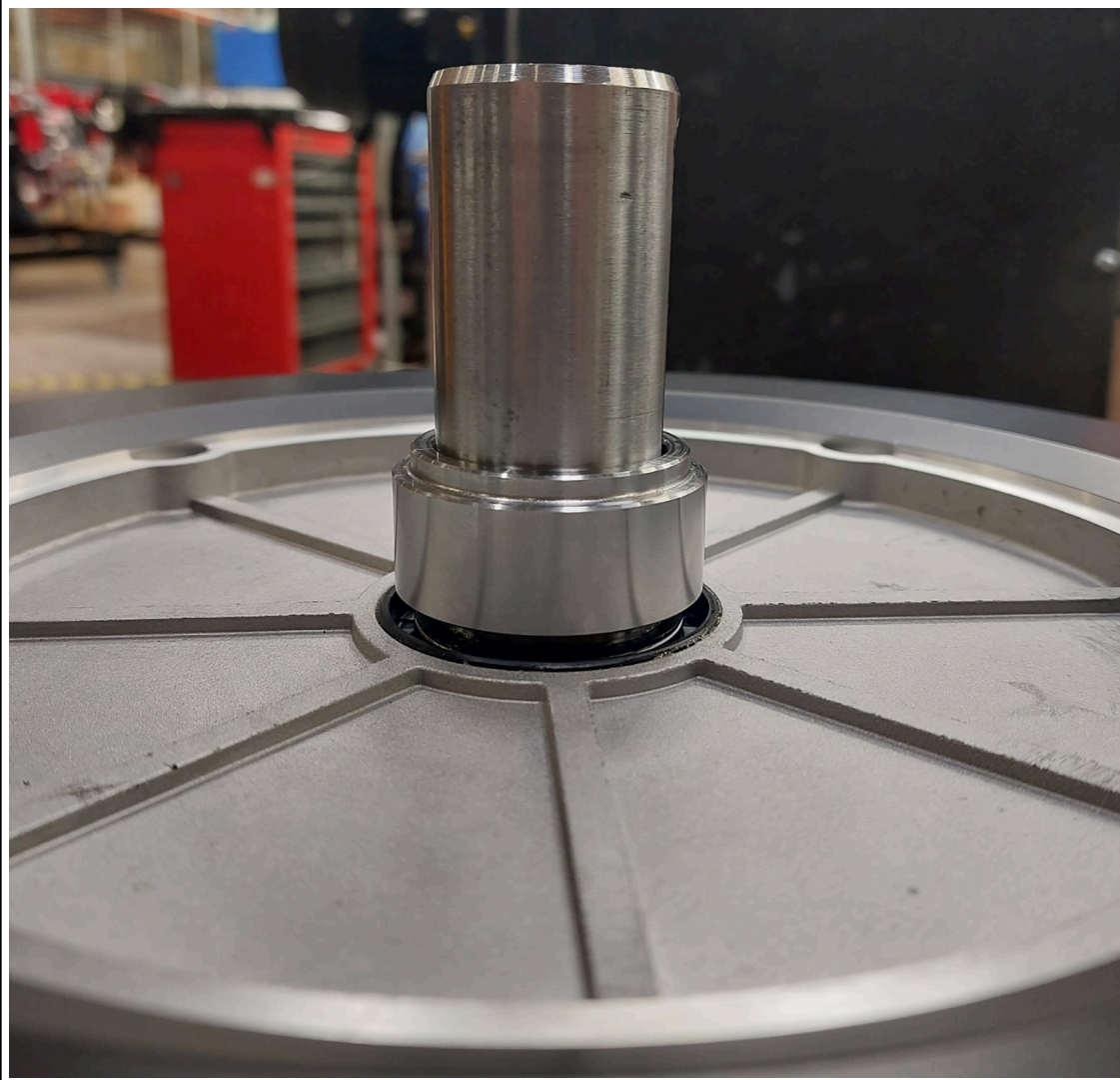
Electric motor and bushing after assembly
