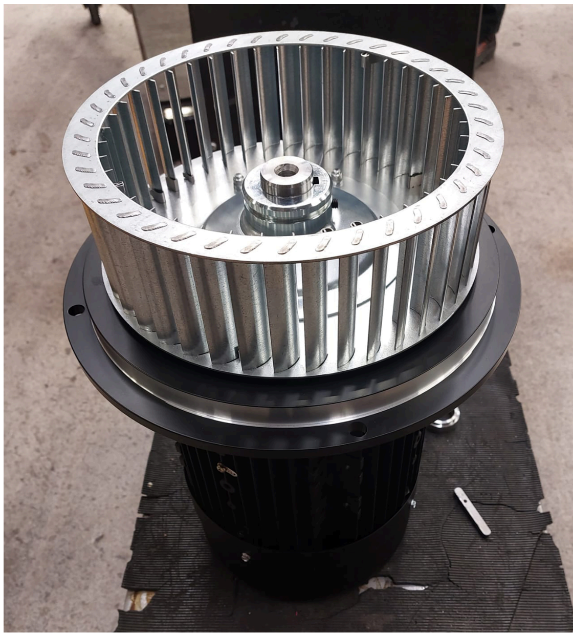
New bushing and reinforced fan wheel assembled
