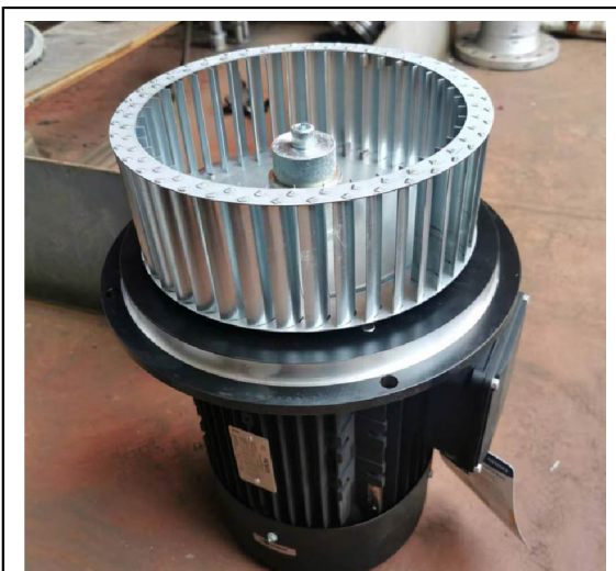
Fan motor assembly on the floor ver. 1
