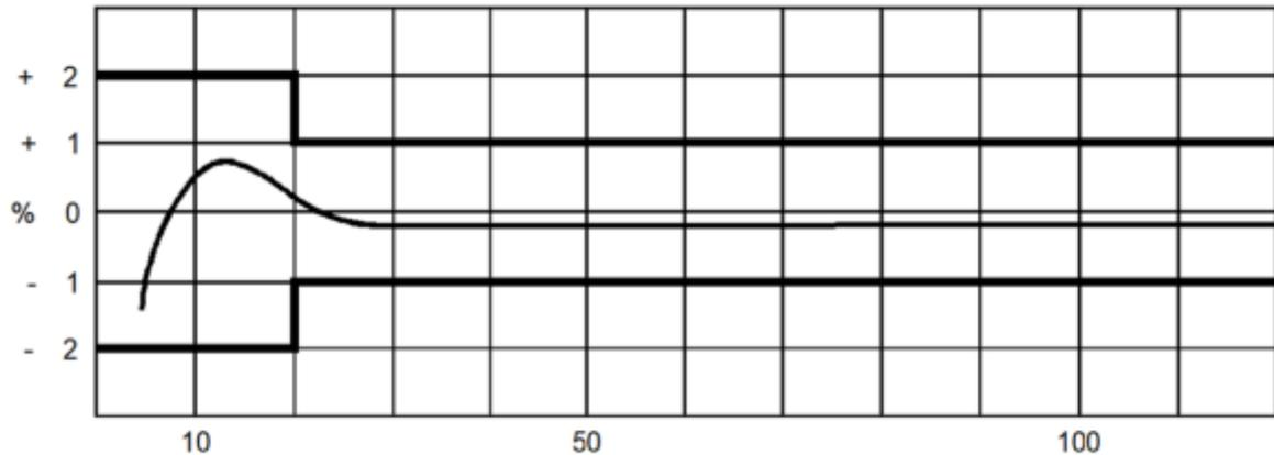
**Figure 2: Calibration curve of a turbine meter**
