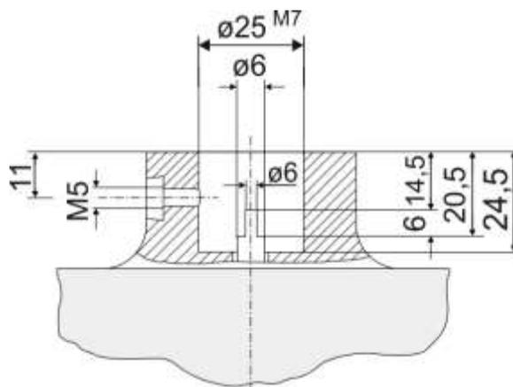
**Figure 8: Dimensions of the drive shaft coupling**
