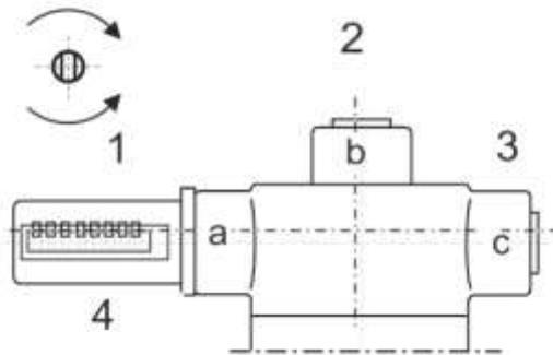
**Figure 7: Direction of rotation of the drive shafts**
