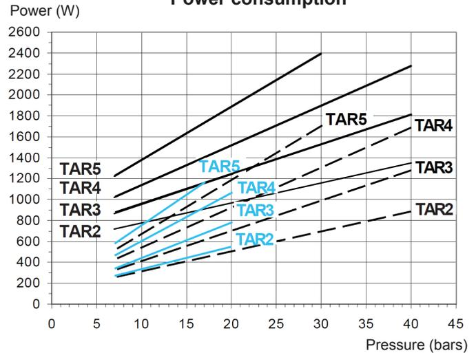
Data shown are for new pumps, with no allowance for wear.
