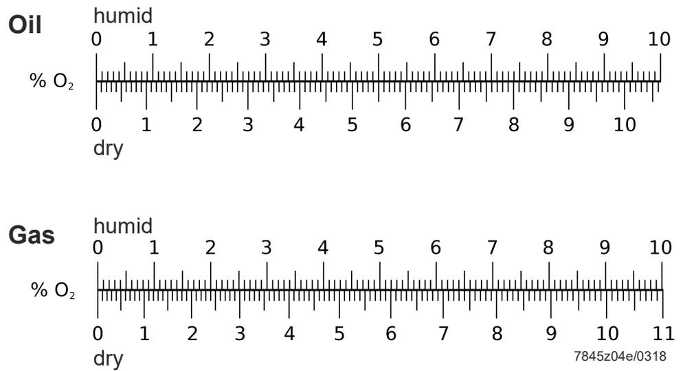
Figure 13: Comparison table for flue gas measurement: Dry/humid
