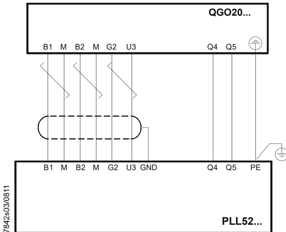
Figure 9: Connection diagram
