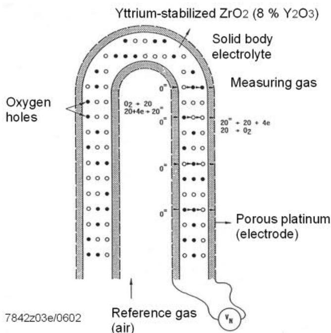
Figure 2: Functioning principle of the measuring cell
