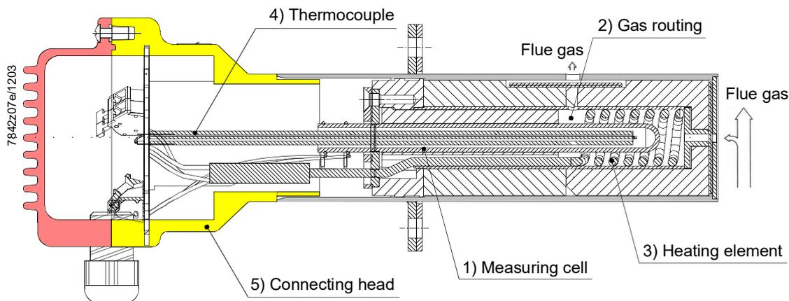
Figure 6: Mechanical design of the oxygen sensor
