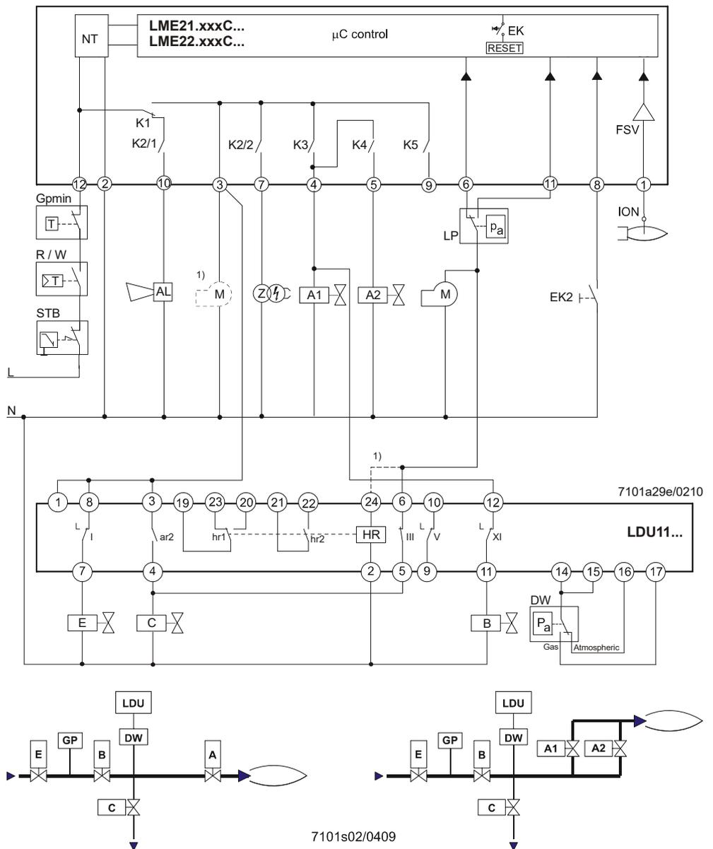
1) In connection with fan motor to terminal 3 of the LME21.xxxC.../LME22.xxxC...
