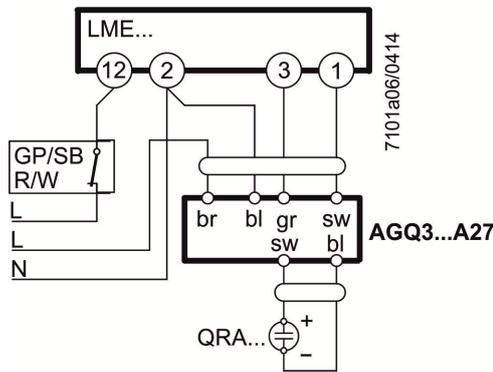
Measuring circuit for measuring the UV flame current
