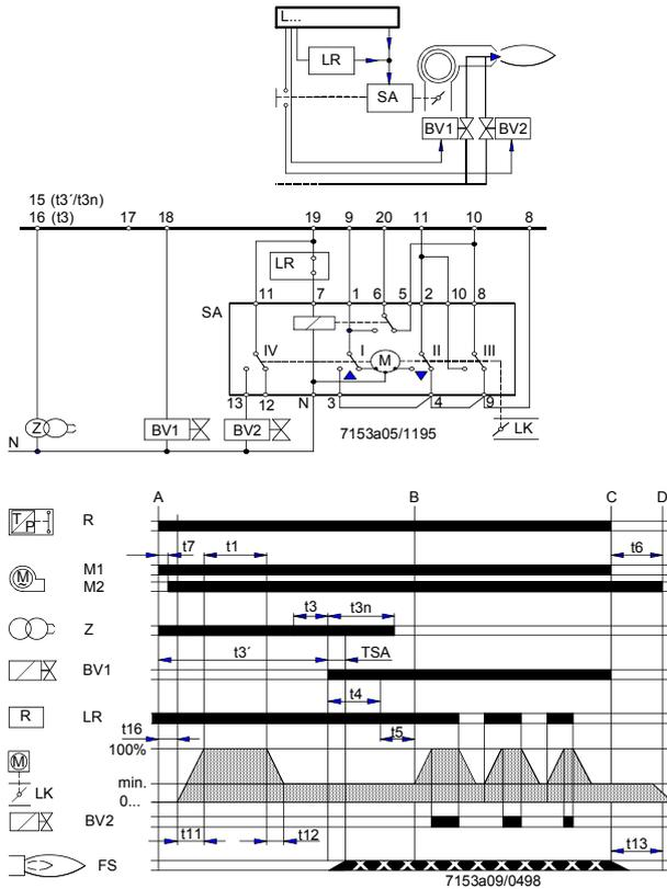
Control of actuator according to the single-wire control principle.
