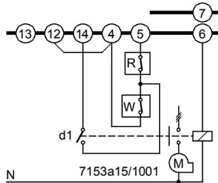
If an auxiliary contact «d1» of the fan contactor is included in the circuit as shown in the diagram, ignition and release of fuel take place only when the contact is closed.
