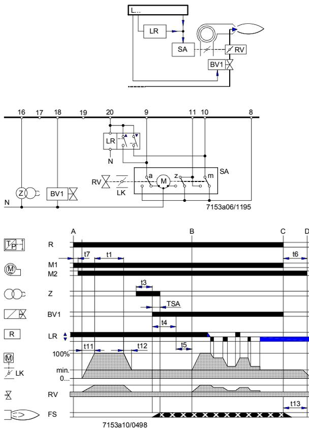
During burner off times, the air damper is fully closed.
