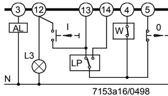
The burner is switched on manually by pressing the «I» button. Then, the LAL programs startup and flame supervision. Burner shutdown is also made manually by pressing the «0» button, or automatically when limit thermostat or pressure switch «W» responds. «L3» indicates when the burner is ready for startup. It extinguishes shortly after the burner is started up. For other connections, refer to «Connection diagrams».
