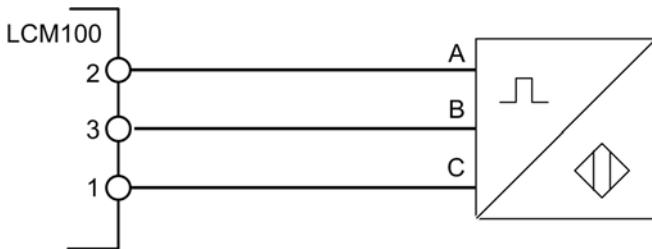
Fig. 8-13 Connection fuel meter for oil with pulse output
