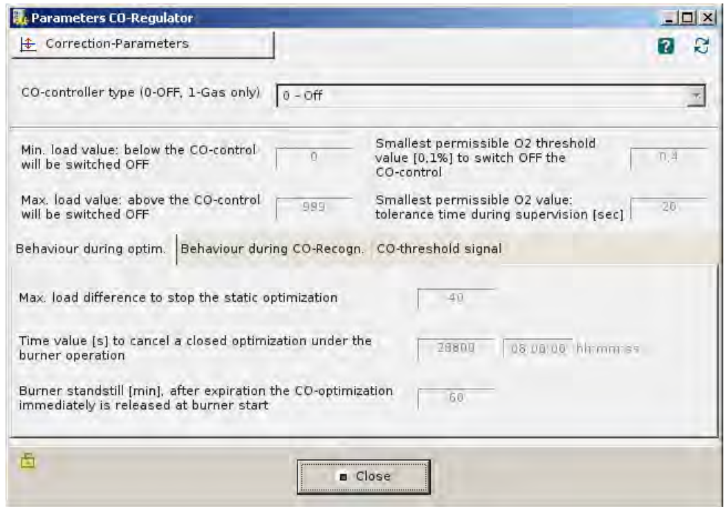
Fig. 6-28 Window for setting CO control parameters
