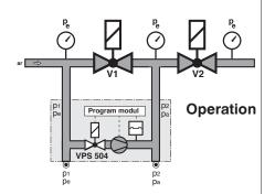
Idle state: Valves 1 and 2 are closed. Pressure build-up: The internal motor pump increases the gas pressure in the test section by approx. 20 mbar compared to the input-side pressure applied to valve V1.
