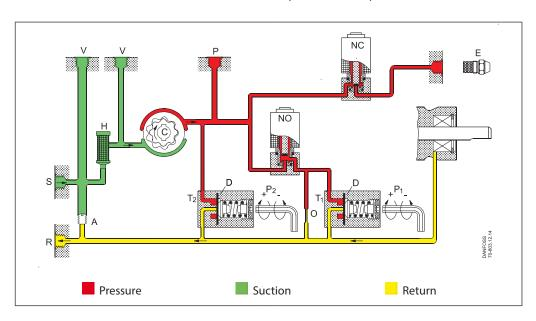
From the suction inlet (S) fuel is drawn through the filter (H) to the gear set, where the pressure is increased. By means of the diaphragm (D) in the pressure regulator for stage 1 ( $T_1$ ), the pressure is kept constant at the value set on adjustment screw ( $P_1$ ).
