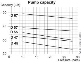
Viscosity = 20 cSt - Rated speed = 2850 rpm
