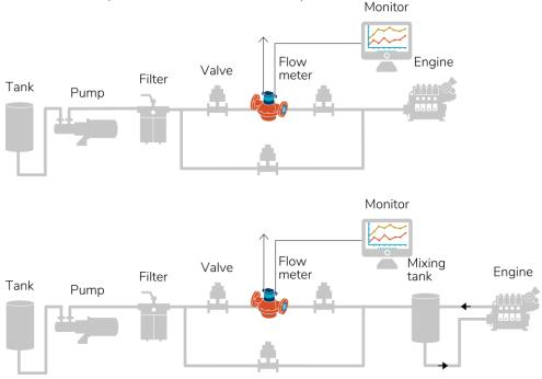
Ship classification societies require the installation of bypass pipes. The relevant regulations must be followed.
