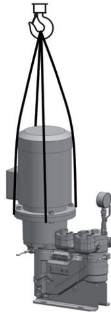
Fig. 10 Fastening the lifting gear to the pump unit vertically or the filter unit with single pump (as illustrated)
