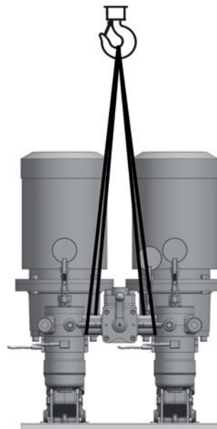
Fig. 11 Fastening the lifting gear to the twin unit with filter
